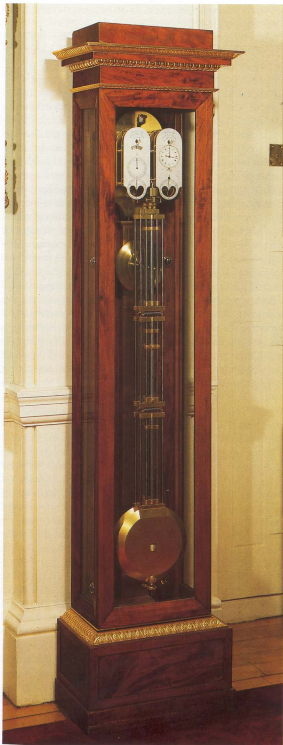
235. (Left) Twin-pendulum regulator by Breguet, general view. (Royal Collection)
