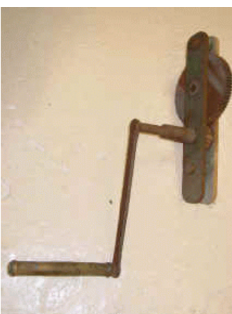
Reduction gear / Winding Jack - Gear system known since antiquity.
