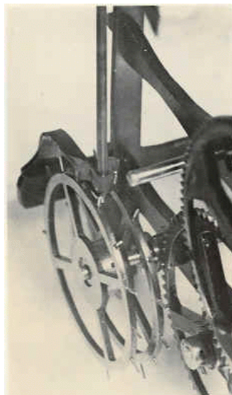
Strob escapement (left) and diagrammatic operation. See next page for discussion.
