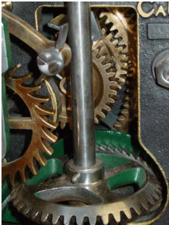
Gravity train remontoire: Epicyclical (planetary gear). George Biddell Airy, England. c. 1860.
