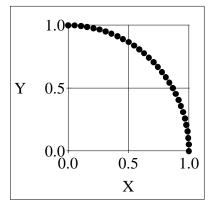
Consider the coordinates of a quarter circle. If you take a horizontal line one inch long and rotate it by one degree at a time until you trace a quarter of a circle, you have points on a drawing which shows the position of each point relative to a horizontal line and a vertical line.
