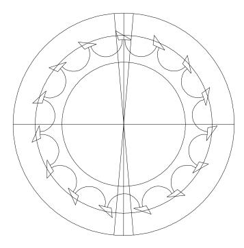
Rotate the tooth in the 7.5 inch circle by 24°. Draw a curve to connect the two teeth by tracing over a small circle. Then draw the escape wheel by duplication and rotation, as before.
