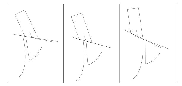
This means that they need not be parallel in the design. If the pallet's impulse face remained unchanged, the efficiency of the escapement would remain unchanged, and we could change the shape of the escape tooth without sacrificing efficiency. The span of the tooth's impulse face could be increased from 2° to 4° so as to draw a wider tooth. The amount of lock would remain unchanged at 3° for the purpose of the drawing:
