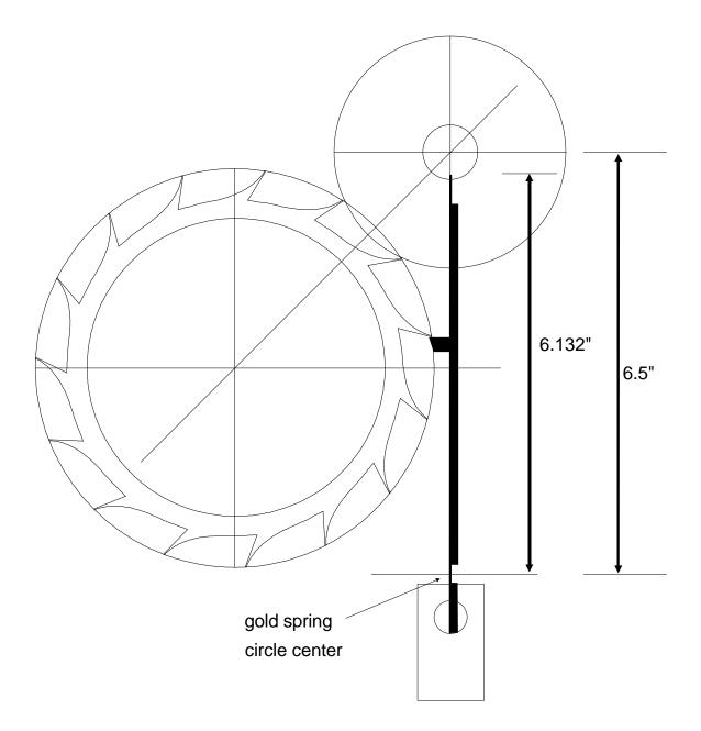
Rotate the detent arm and gold spring assembly clockwise by 1°, until the detent pallet just releases the escape tooth. Rotate the discharge pallet counterclockwise by 8°. Draw the impulse pallet at the edge of the impulse pallet's circle, just inside the escape wheel's circle.
