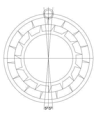
The impulse arm's length could be found by trial and error, or it could be calculated. In this example, the impulse arm rotates by 60° during impulse. The escape wheel rotates by 24°, less 2° for drop, or 22°. The impulse arm's circle radius will be given by 'X', and the inner escape wheel's circle radius by 'W'.
