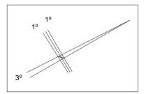
If you rotate line (2) counterclockwise by  $2^{\circ}$ , you would see that the escape wheel's impulse face occupies a span of  $2^{\circ}$  of escape wheel rotation. (The impulse face also provides  $3^{\circ}$  of lift and lock.)
