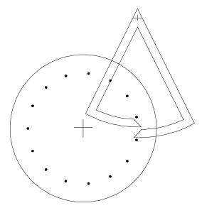
Changing the pallet circle's diameter does not affect the number of teeth between the pallets, as it does in the Graham. However, it does affect the angle of swing of the pallets (from side to side). If the pallet circle radius were increased, the angle of swing could be decreased, which is desirable for a fine regulator. This would make it possible to minimize the circular error in the movement of the pendulum.
