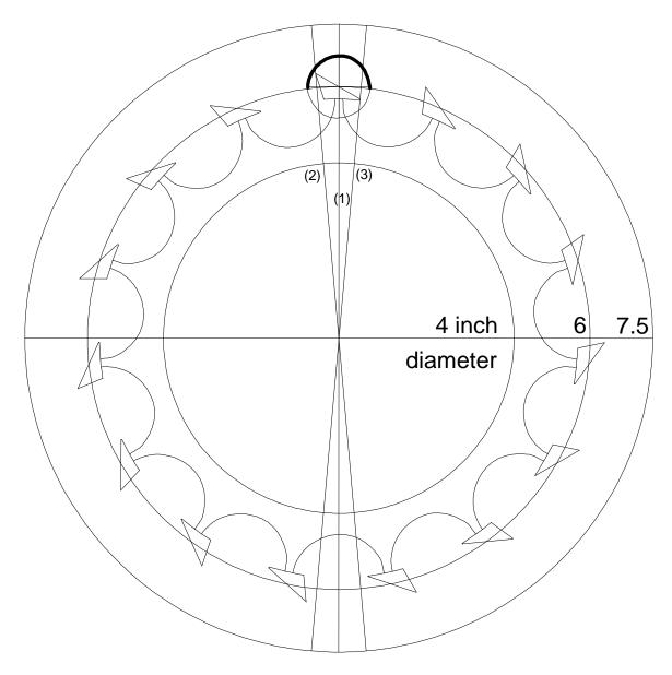
Increasing the diameter of the cylinder circle results in a proportional increase in the inside drop and an equal decrease in the outside drop.
