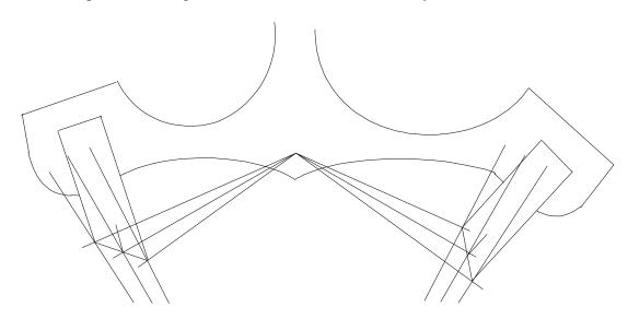
This was not mentioned in Chapter 15 in order to focus attention upon the need to maximize the efficiency of the impulse face angles. The result is two *identical* pallets with impulse face angles as close to 45° as possible.
