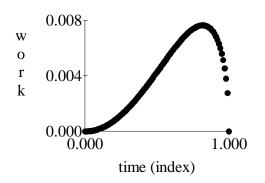
The impulse face's angle changes unevenly over the time it takes the escape tooth to pass over the impulse face. If you consider the *displacement* (or distance moved) of the pallet in the direction of Fp, and multiply this by the *force* Fp that rotates the pallet at each instant in time, you get a 'work done' curve. This curve looks very different and reveals how inefficient the Brocot design really is.
