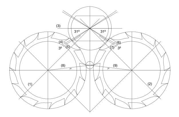
The upper locking pallet should have a width equal to the gap between the escape wheels and should have a "V" shape to allow for a draw angle of 10°. Place the pallet 7° above the horizontal line, shown by the point where lines (8) and (9) intersect.
