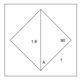
Draw two triangles using this arrangement:  $\cos (A) = 1 / 1.6$   $A = a\cos (1 / 1.6) = 51.3^{\circ}$ Use this to determine the tooth span: 30 x (2 x 51.3 / 360) = 8.553so you should use a span of 8.5 teeth.
