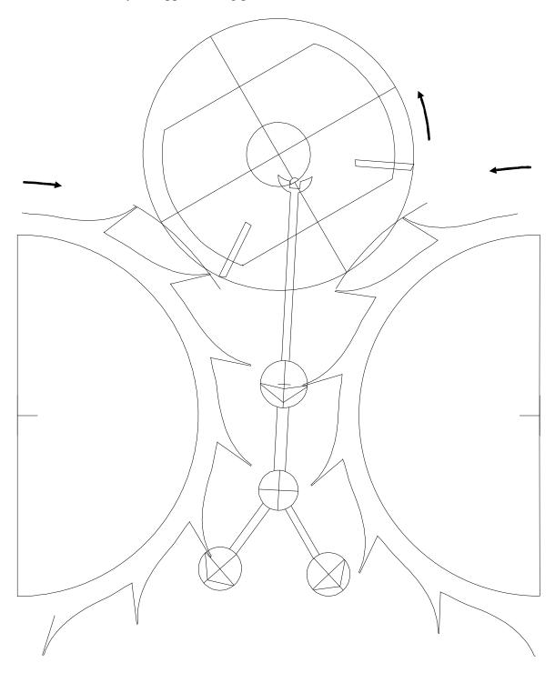
The drawing on the previous page reveals how complicated the design is. Notice how the escape wheel and the impulse pallet appear to *roll* together, instead of sliding across one another, and therefore why the escape wheels and the pallets need not be lubricated.
