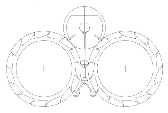
In this drawing, I have rotated the locking pallets clockwise by 3° and the impulse pallet / roller table assembly counterclockwise by 30°. The left escape wheel has just been released by the impulse pallet and is detained by a lower locking pallet. The right escape wheel is detained by the upper locking pallet.
