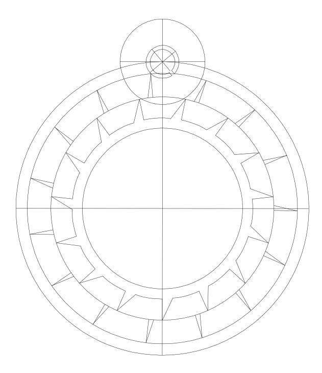
Rotate the escape wheel clockwise by 12°: in other words, 2° after the tooth has been released by the locking jewel. Rotate the locking jewel until it is at the point where it has just released the escape wheel's tooth. Then draw the impulse arm next to the inner escape wheel's tooth in its path.
