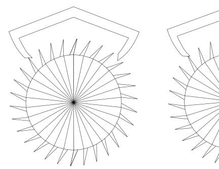
Be aware, when you prepare to do a simulation, that the group of lines comprising the pallets and the escape wheel must be symmetrical about the point you intend to rotate, because if the center of the group were not the same as the center of the pallets, for example, then the rotation would not take place the way you want it to. Therefore, the circles should be included in the groups being rotated, as shown in the drawing that preceded the simulation.
