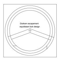
If the pallets were modified to make them with equidistant lock, the locking faces would be drawn on the same circle. However, the pendulum would receive unequal impulses in each direction. A pallet with equidistant drop could similarly be designed, but it has no practical application in horology.
