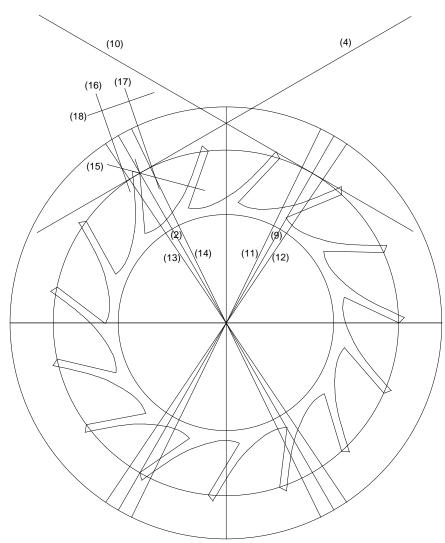
Once you finish the entry pallet, group the lines and duplicate them. Rotate the second pallet clockwise by  $60^{\circ}$  because that is the angle between lines (2) and (9), and then place the pallet on the exit side such that the mid-point of the impulse face lies on the point where lines (9) and (10) intersect. Most watches have different pallets, but an escapement using the same pallet on both sides can be designed, and using the same pallets makes manufacture easier.
