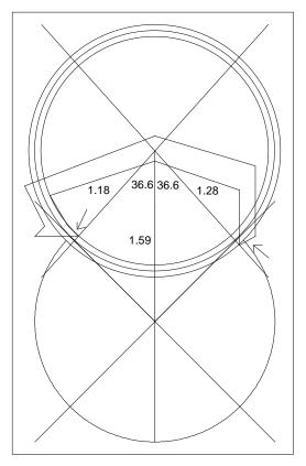
For the radius calculation, decrease the pallet radius on the entry pallet by the amount of a quarter of the arc between two escape wheel teeth, and increase the pallet radius on the exit pallet similarly. This is only a close approximation because the change in the pallet circle's radius is assumed to be equal to the arc of the escape circle, but an arc is not a straight line.
