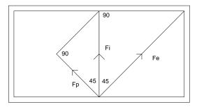
If the angle of the pallet's impulse face were changed, the direction of Fi would change, and therefore the proportion of Fe that could be used to rotate the pallet: could be used to create this:
