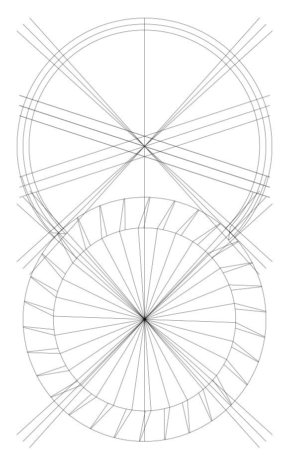
During the simulation, the escape wheel and the pallets are rotated by one degree at a time in their respective directions.
