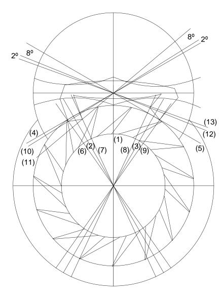
Rotate line (6) clockwise by 15° to get line (14), which will be the entry pallet's locking face with a draw angle of 15°. Duplicate line (14) and place it on the point where lines (7) and (11) intersect. Repeat this procedure for the exit pallet: rotate line (8) clockwise by 15° to get line (16). Duplicate line (16) and place it on the point where lines (5) and (9) intersect. Finish the drawing as you wish.
