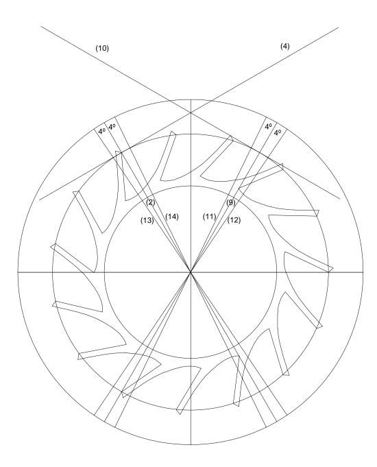
Rotate line (2) counterclockwise by 45° to get line (15). Notice that it is at an angle half way between the escape circle's radius and the pallet circle's radius, shown by lines (2) and (4) respectively:
