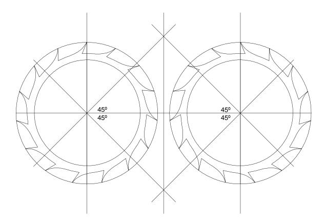
You need to find the radius of the impulse pallet's circle (X), as for the Chronometer. If the escape wheel rotates  $18^{\circ}$  (24° less 3° *twice* for drop) during impulse, you could draw the following triangles:
