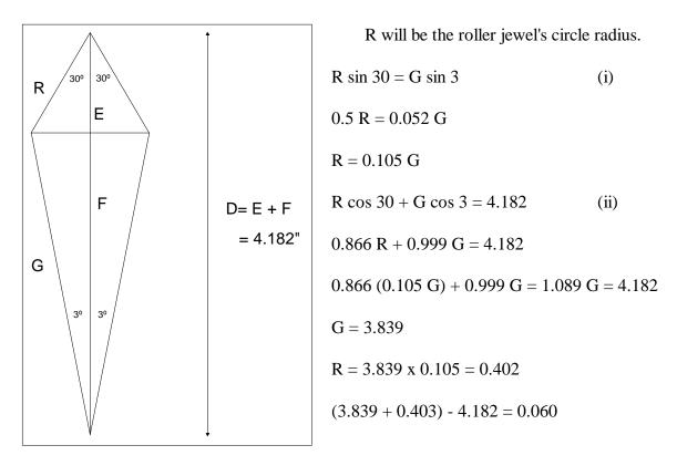
Draw the roller jewel's circle with a radius of 0.402 inches, and place it such that its center lies on the center of the impulse pallet's circle. Draw the pallet fork with a radius of 3.839 inches from the locking pallets' circle center to the entrance corner of the fork horn: the roller jewel would have a depth of 0.06 inches inside the pallet fork. I have not included the locking pallets' circle in this drawing, but it would be needed for a simulation.
