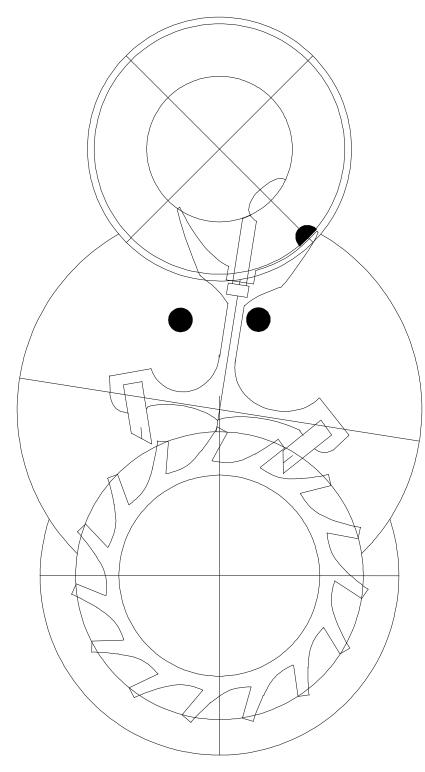
Rotate the pallets until a tooth is released: this is the "drop-lock position." Rotate the roller table until the safety notch is just beyond the guard pin, which appears to be pressed against the safety roller. Draw the fork horn just outside the path of the roller jewel, and extending to the jewel's other side, as shown. This design prevents premature unlocking. Repeat on the other side.
