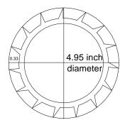
The inner escape wheel has smaller teeth, but they are similar and also have perpendicular locking faces. Draw it in a 4.95 inch diameter circle, each tooth having a height of a third of an inch. Both escape wheels need to be designed so that they could be rotated either together or independently.
