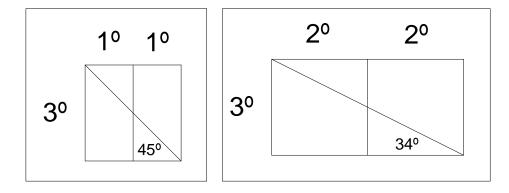
If the escape tooth occupied a span of 4° and there were 2° of drop, the pallet would occupy a span of 6°, for a total span of 12° per beat. New pallets must be drawn.
