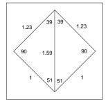
Assume a small error in measurement:  $\cos (51) = 1 / h$   $h = 1 / \cos (51) = 1.59''$ The pallet angle is : 180 - 90 - 51 = 39° The pallet circle radius is:  $Rp = 1 x \tan (51) = 1.23$
