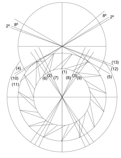
The 15 tooth escape wheel rotates by  $12^{\circ}$  per beat, so make the pallet occupy a span of  $10^{\circ}$ , in order to allow  $2^{\circ}$  for drop.
