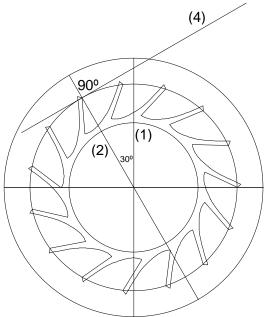
The first tooth was drawn next to line (2), which had an angle of  $30^{\circ}$  relative to the vertical line (1). The  $30^{\circ}$  angle was chosen so that there would be a 2.5 tooth span between the pallets for a 15 tooth wheel. The angle between lines (2) and (4) was 90° so that the angle between the force exerted by the escape tooth and the force that acted to rotate the pallet would be 90°.
