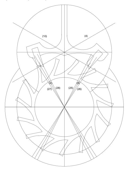
Another way to make a stronger tooth would be to trace the path of the pallet during the simulation, and then to draw the curve on the back side of the tooth again. If the simulation were superimposed for the action of the escapement as the tooth pushed on the entry pallet,
