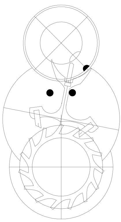
guard finger were too long, there would be no gap between the guard finger and the safety roller when the fork is pressed against the banking pin. This gap is called "guard finger freedom."
