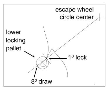
tooth, as shown below, giving the pallet 1° of lock and a draw angle of 8°. Notice that the sum of 10° for upper draw and 8° for lower draw gives 18° for total draw: this is similar, if only slightly more than the 15° for draw designed into the Swiss Lever pallets.
