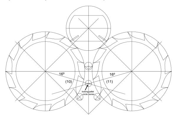
Before drawing the roller jewel that moves the locking pallets from side to side, you need to find the distance from the roller jewel's circle center to the locking pallets' circle center. I will call this distance "D."
