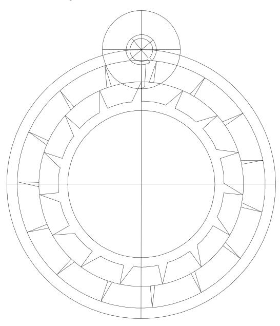
By analyzing the drawing, you would find that the escape wheel provides a considerable impulse during the locking phase, not only during the impulse phase.
