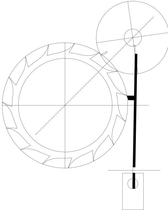
Rotate the detent clockwise by 1° extra, and the discharge and impulse pallets counterclockwise until the discharge pallet meets the gold spring. Then rotate the escape wheel until it meets the impulse pallet. The discharge and impulse pallets must rotate by enough to allow the escape wheel to move forwards until the tooth clears the detent before the detent is released. Otherwise, there will be some bent escape teeth.
