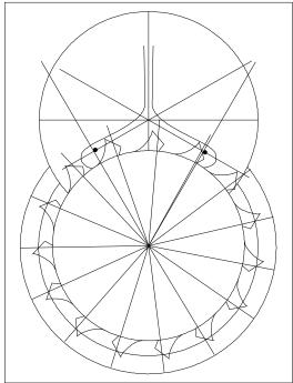
Since clocks do not have pallets that are independent from the pendulum, there is *no need for draw*. Therefore, the equidistant lock design is of no advantage in pendulum clocks. The equidistant impulse design is the obvious choice for the Graham, Recoil, and Brocot escapements. (It cannot be applied to the Pin Wheel escapement, as its drawing demonstrates.)
