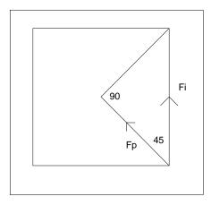
As the pallet is pushed by the tooth, it rotates clockwise, so a portion of Fi is received by the pallet to push it in a North-West direction.
